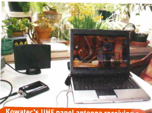
Kowatec's UHF panel antenna receiving a telenovela from WUVP-66.
